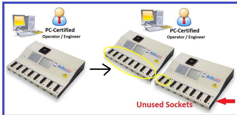
Conventional 8-gang programmer - costly setup during project expansion.
