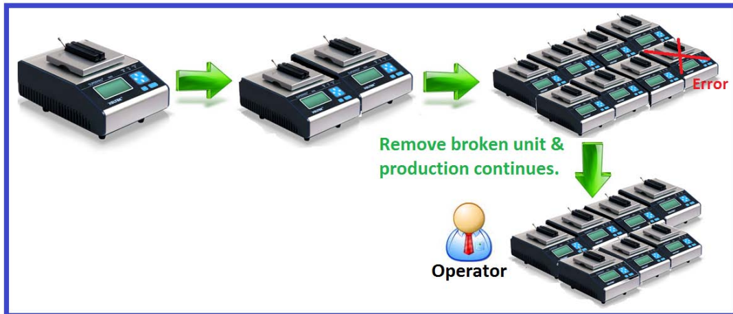
SuperPro® Stand-Alone programmer solution for defective units during manufacturing.
