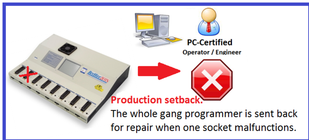
Conventional gang programmer set up is not practical when one socket is defective.
