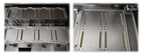
On the left is the SB05 applicable programmer group, divided into two groups before and after, a total of 8 modules, through the 8usb line alone communication.
