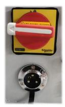
The red knob above is the load switch which is on the back of the machine, after opening the system is on power.
