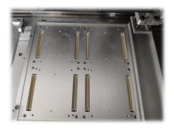
This is the programmer group for SB04, and the 4 module is centralized to 1 USB cable communications via the hub board.
