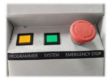
Programmer: Button controls the power supply of the programmers.
