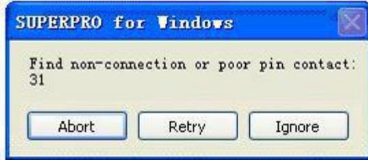
If the chip has been inserted, the pin contact is poor or some pin(s) of the chip has been damaged.
