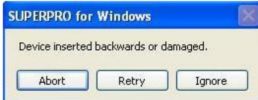
The chip has been inserted backwards. Please take out the chip, reverse it and insert again properly. If the problem still exists, the chip may have been damaged.
