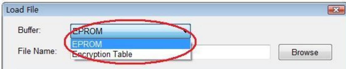
2. To select a data file to be loaded, the path and the file name should be entered into the name field. You can directly input the file name or click the “Browse” button to select the file in the Select File box.
