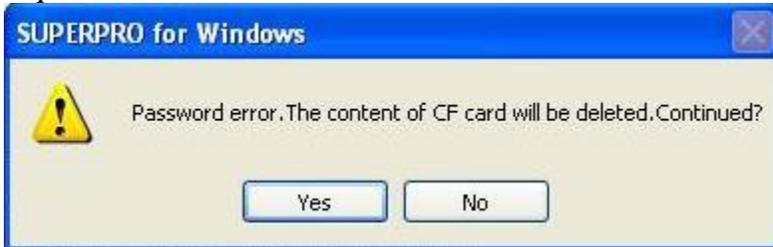
Password error. The data in the storage module (CF card) will be deleted permanently. Select 'Yes' to continue.
