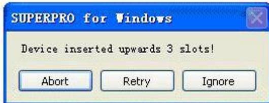
The chip has been inserted improperly. It has been inserted upwards. Please refer to 'Device Insertion' in the manual.
