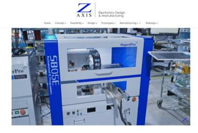
May 14, 2021 - Z-AXIS Inc. (www.zaxis.net) has added a Xeltek SuperBOT 5e robotic IC (integrated circuit) programmer at its electronics design and contract manufacturing center near Rochester, NY. The \$80,000 robotic system replaces an earlier model, processing ICs three times faster and reliably handling the latest fine-pitch IC packages.
